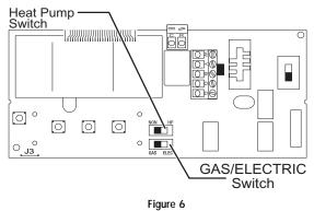
17. A temperature limiting jumper has been included in this thermostat. Cutting this jumper (J3) limits the heating setpoint to no greater than 72°F and the cooling setpoint to no lower than 78°F (Figure 7).
